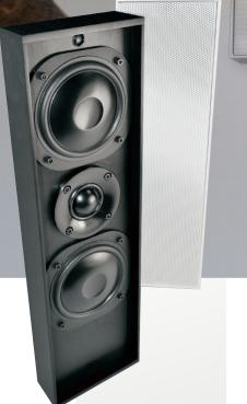
Size 14 h x 4 w x 1.5 d (in) 355 h x 101 w x 38 d (mm) Freq Response 90Hz-22kHz±3dB Impedance 8 ohms Sensitivity 86dB 2.83V /1m Power req. 25 -100 watts Woofer (2) 3.5" (89mm) Aluminum (Active/Passive) Tweeter (1) 1" (25mm) Soft Dome Mount Through hole (Optional Brackets) Finishes Gloss White, Satin Black, or Custom
