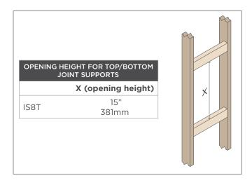
Place space saver, preconstruction zip ring bracket, or both in desired speaker location. See page 5 for when to use space savers and zip rings. Space savers are recommended for every new construction project. Zip rings are recommended as a time-saver on very large projects with dozens of invisible speakers.
