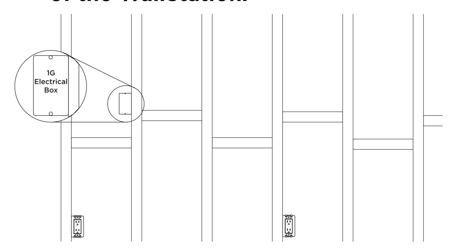
NOTE: The CONNECT PRO WallStation will cover a 1G electrical box only. A 2 Gang electrical box will interfere with the mounting hardware.
