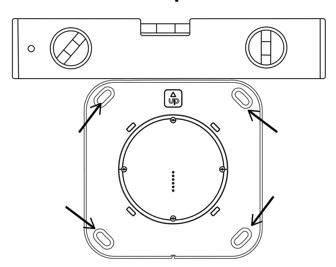
4. Remove the WallStation form the wall once you have marked the 4 anchor locations.
