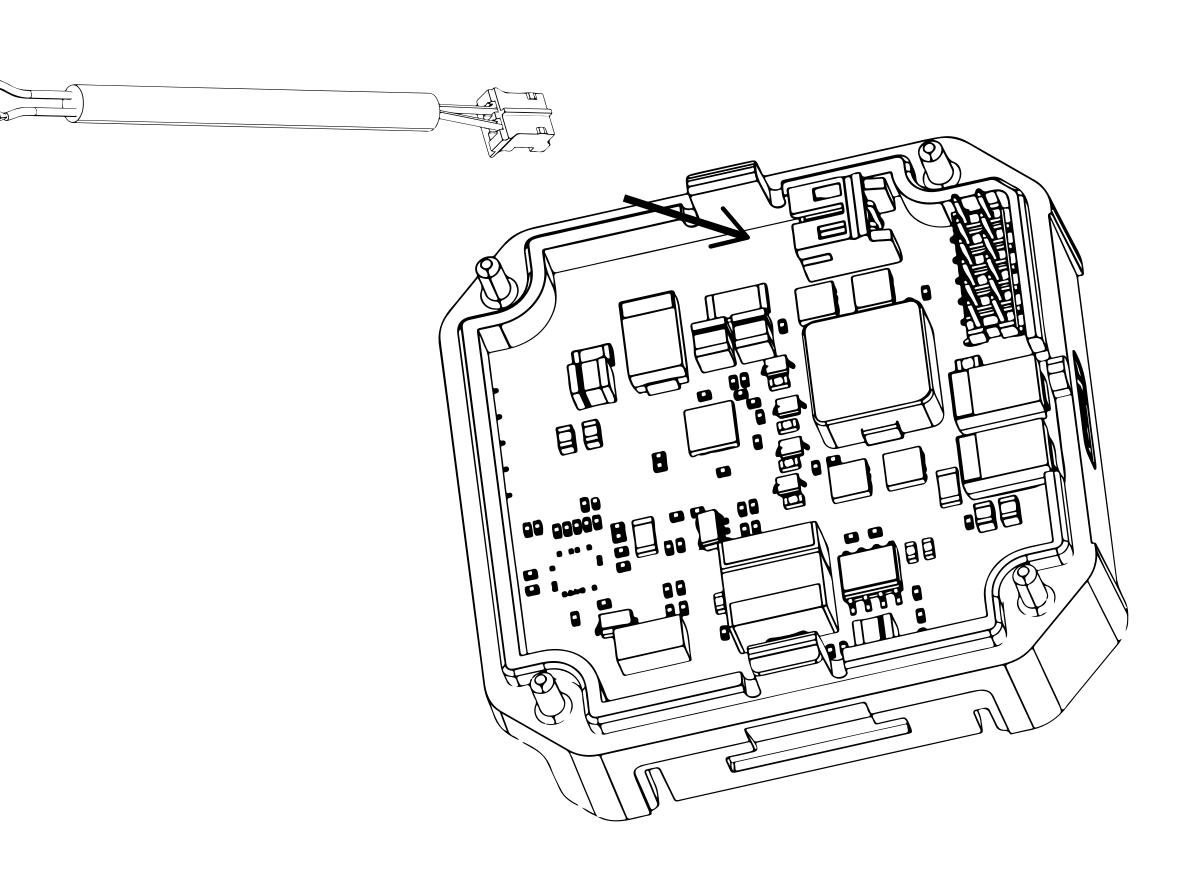
Zip tie the Connector to the DC board for added cable retnetion.
