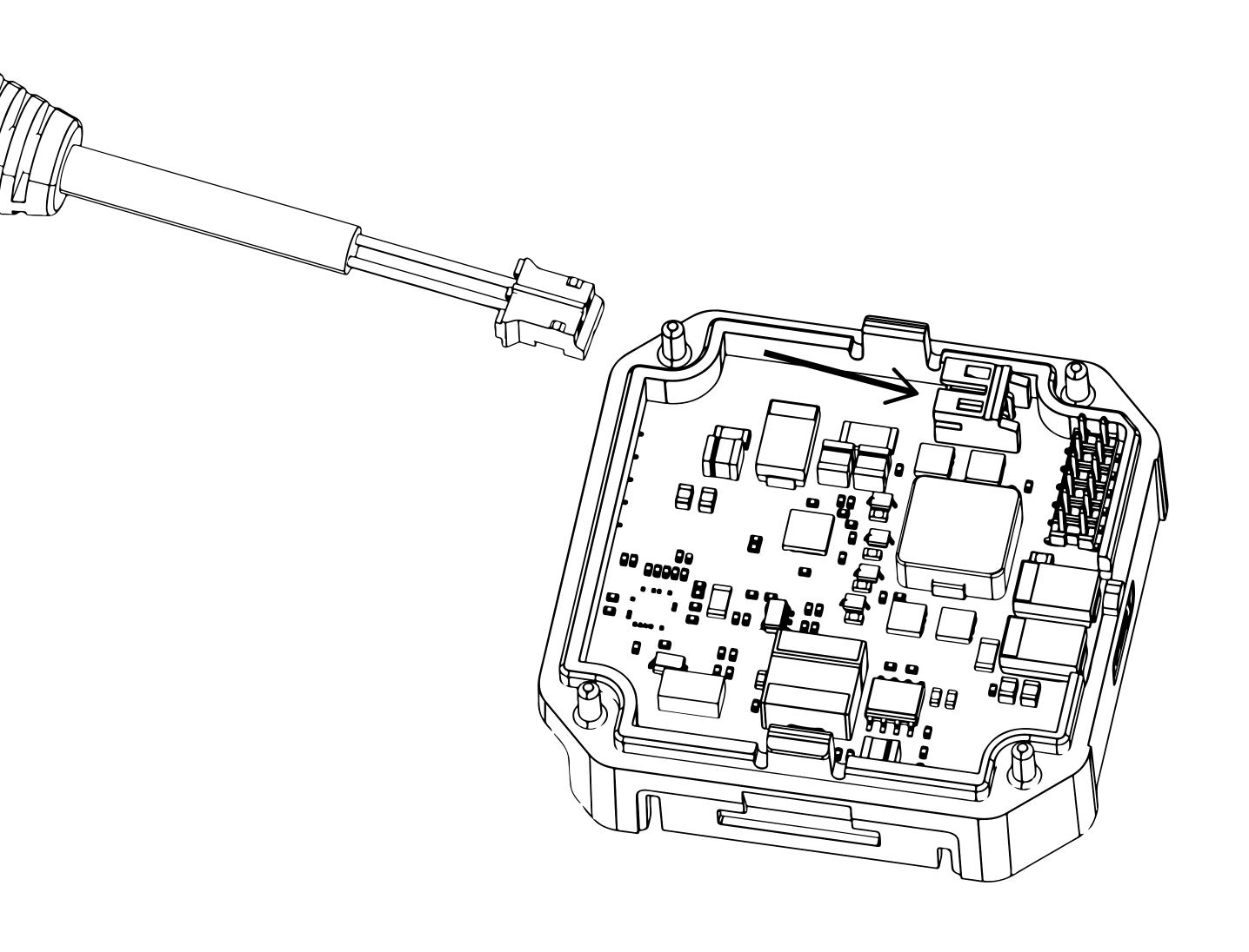
Zip tie the Connector to the DC board for added cable retnetion.
