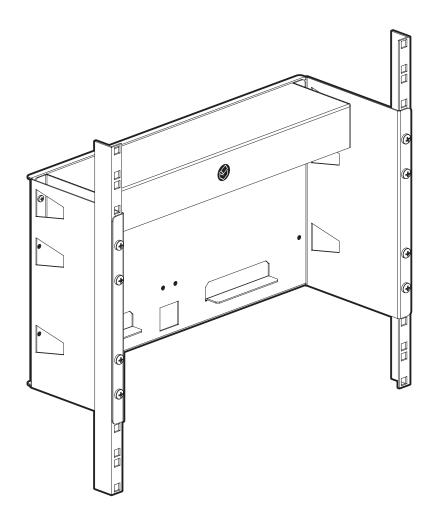
The S7 NetAmp 19" Rack Adapter allows installation of two NetAmps onto a 6U adapter. The NetAmp wall brackets are used to mount the NetAmps. The adapter also includes a cable tidy box which can be mounted when all the connections have been made. Cable entry points have been made at the top for the main connections and at the bottom for the power cable. The adapter is only 150mm deep allowing two to be mounted back to back on the rack if accessible, 6U then accommodating 8 zones.
