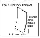
To remove the peel and stick plate, pry up the bottom and pull/stretch the adhesive strip downward.
