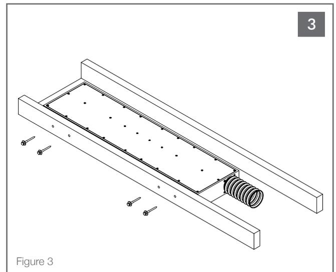
Hold the side of the BPS6 TL Subwoofer with the rubber damping pad up against the side of the stud or joist and install the four lag screws and washers to secure the BPS6 TL Subwoofer in place. (See Figure 3).
