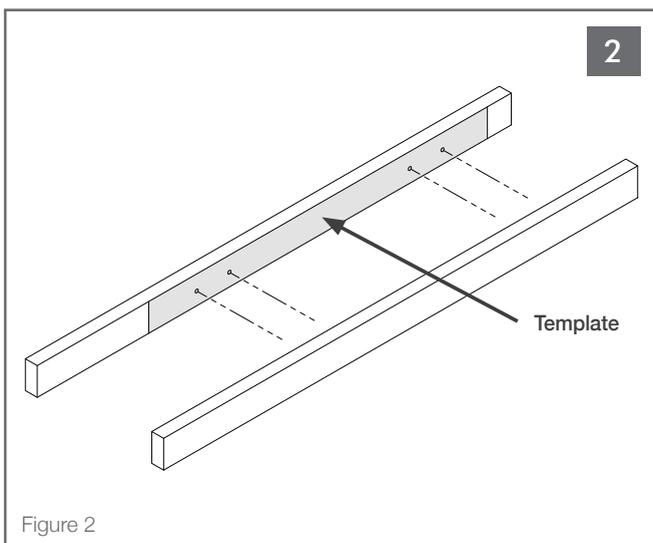
Place the subwoofer mounting template on the side of a 2 x 4 stud or joist and drill four 1/4" (6mm) holes through the stud at the locations shown on the mounting template. (See Figure 2).
