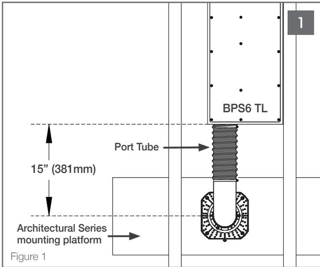
Determine the location of the mounting platform and subwoofer. Ensure there is adequate space to accommodate the subwoofer and port tube within the 2 x 4 stud bay or joist, allowing 15" from the front edge of the BPS6 TL to the center of connector. (See Figure 1).
