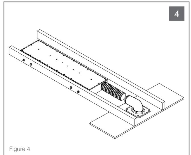
Prepare to attach the mounting platform to the stud or joist. Position the platform with the 90 degree connector pointed in the direction of the BPS6 TL port tube. (See Figure 4).
